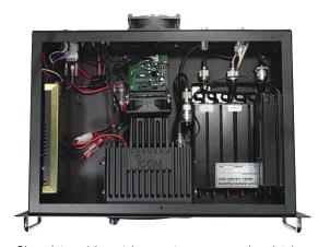
Clean internal layout is easy to access and maintain. Repeater, duplexer, pre-selector and power supply, all in one box.
